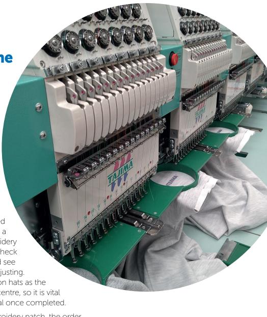
The embroidery machines are manually threaded with the colours of your design. The machines can use up to 12 colours at a time! Thread colours can't be pantone matched, but there is such a huge array that we can usually get quite close.
